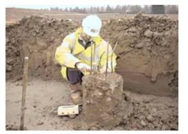
Pile Integrity Testing (PIT)
